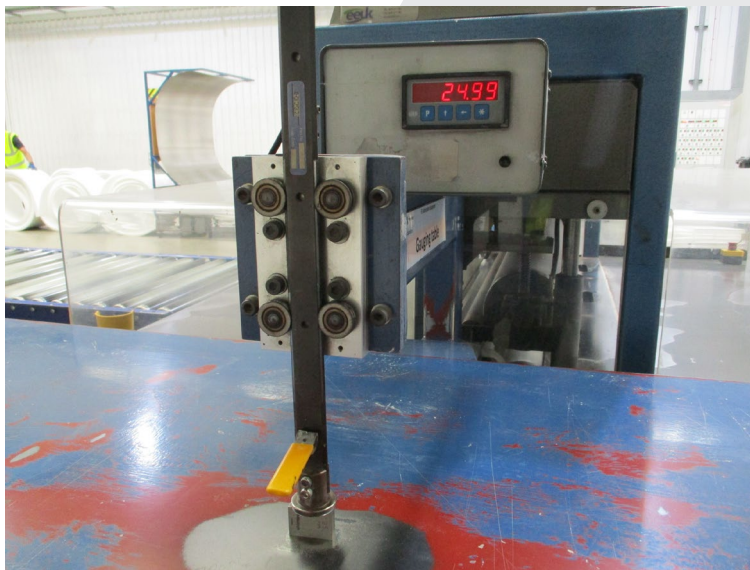
Figure 7 Calibration of gauge table using a 25mm gauge block
