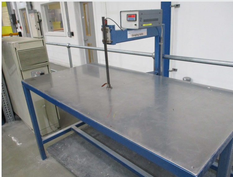
Figure 1 Side view of thickness gauge on gauging table
