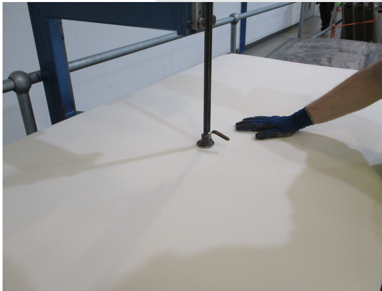
Figure 5 Centre thickness measurement
